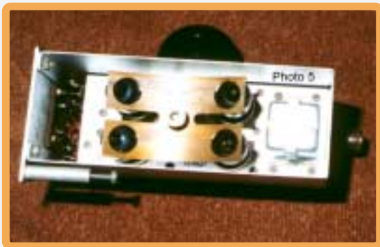
Photo 5 - Amplifier module - tube side
