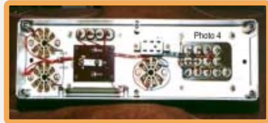
Photo 4 - Underside of the power supply chassis
